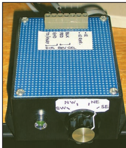
Figure 6 — A rotary switch allows the operator to select the appropriate antenna and direction with a single control. BEV refers to the antenna select relay and DIR to the RBS-1 direction control.
